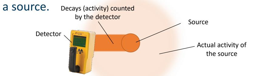
To count all the radiation emitted, a detector would need to completely surround a source.
